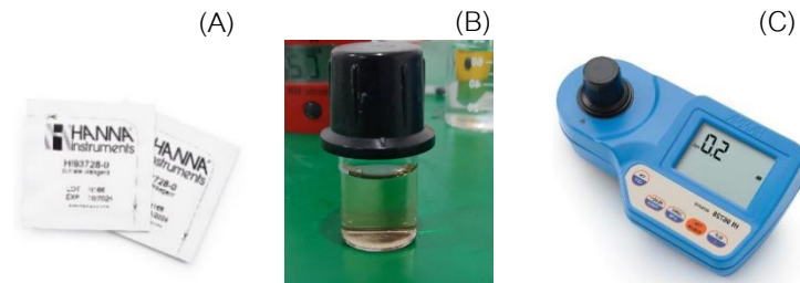
Fig. 1 Process Measurement of Concentration of Nitrate (A) Cadmium Reagent (B) Water Sample Color Changed to Yellow (C) HANNA Nitrate Portable Photometer
