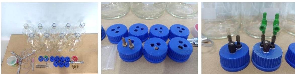
Fig. 2 Equipment for Biochemical Methane Potential Test (BMP)
