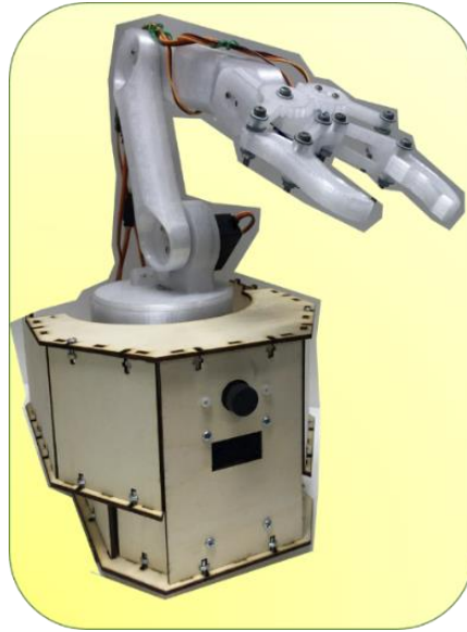
Fig. 2 Robot Arm 6 axis with OpenMV Camera
