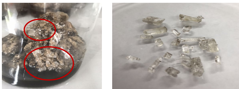
Fig. 2 The crystals from waste latex sludge digestion using sulfuric acid
