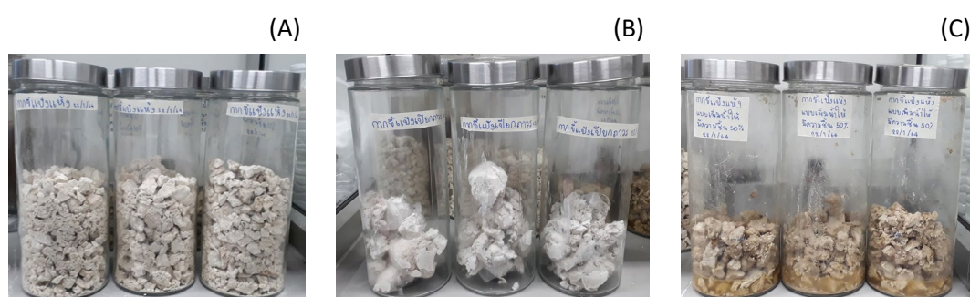
Fig. 1 (A) waste latex sludge dry, (B) waste latex sludge wet, and (C) dried waste latex sludge soaked in water
